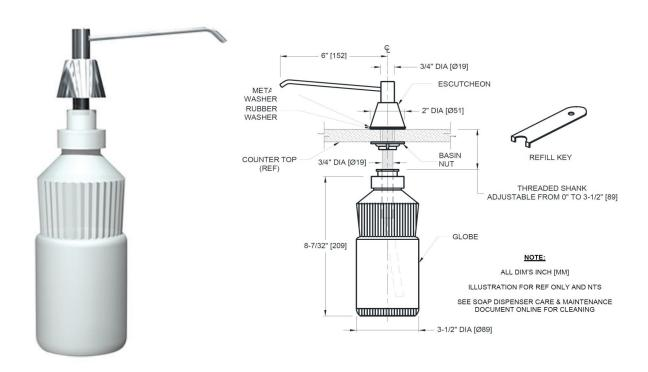
Model WA0332-D is our countertop liquid soap dispenser, designed for deck mounting. Supplied with a 0.9 litre capacity polyethylene liquid soap reservoir to be mounted below countertops. All liquid soaps should be chloride free and pH neutral. Requires 25mm diameter hole in countertop positioned so that the spout swivels to direct soap outlet over sink or bowl.
